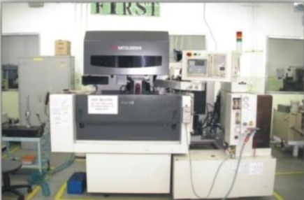
WIRE CUT MACHINE (MITSUBISHI FA10S)
