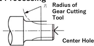
Note that a step near gear may interfere with the gear cutting tool on its cutting.
