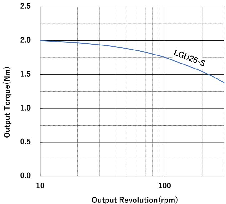
※The torque curve of the final stage(output side) is described.
