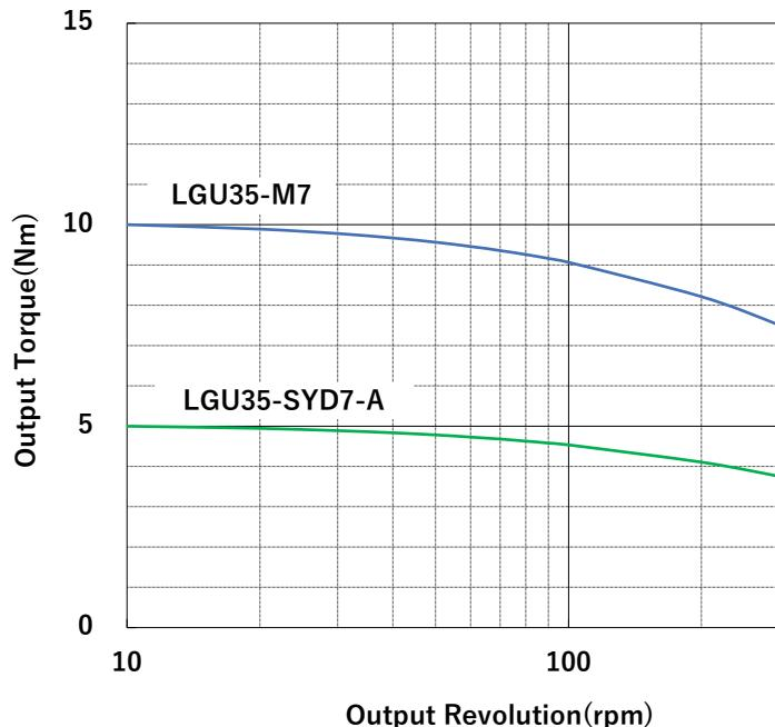
※The torque curve of the final stage(output side) is described.
