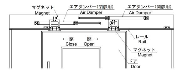
To fix the air damper body, screw the four slot holes. Use screws with sufficient length for fixing screws.
