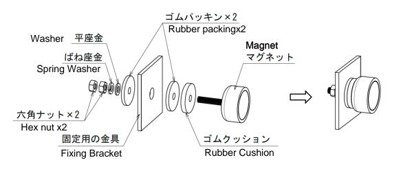
To fix the magnet, hold the fixing bracket between the two rubber packings as shown above. Also, before use, tighten the two hex nuts sufficiently and check that they are not loose.
