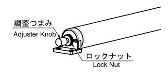
Adjust the damping force after loosening the lock nut. Tightening the adjustment knob clockwise will increase the damping force, and loosening it counterclockwise will decrease the damping force. After adjustment, tighten the lock nut before use.
